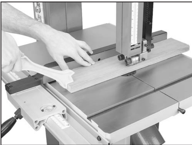
Figure 32. Typical ripping operation.
